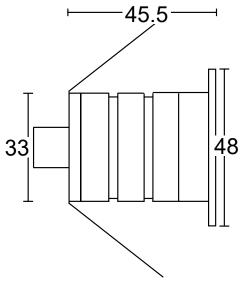
TD011 is a round 12-24V DC deck light, the housing is 6063 anodised aluminium with a stainless steel faceplate. It is IP67 rated, with an Epistar 3W COB chip.It is designed to be recessed into decks or walls and soffits as walk-way lighting.
