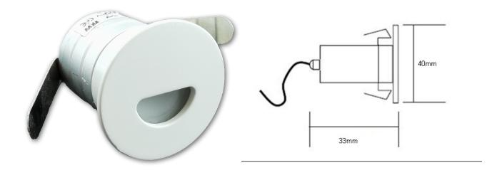
TD018 is a round 12-24V DC deck light, the housing is 6063 white aluminium. It is IP66 rated, with a 1W Cree high power chip. It is designed to be recessed into decks or walls and soffits as walk-way lighting.
