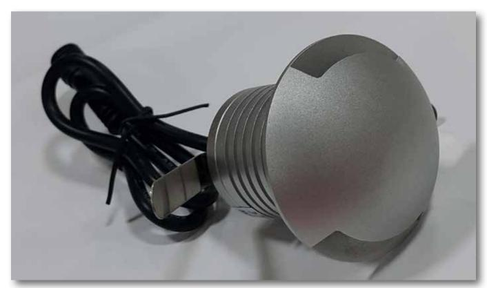
TD013 is a rounded 24V DC deck light, the housing is 6063 anodised aluminium with a double slot. It is IP67 rated, with an Epistar 3W COB chip. It is designed to be recessed into decks or walls and soffits as walk-way lighting.
