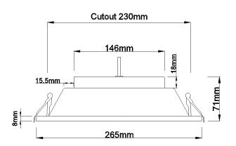
This fitting was designed for and installed in the Selwyn District Council Building to replace their exisiting fittings, eliminating the need for remedial work on the ceilings.
